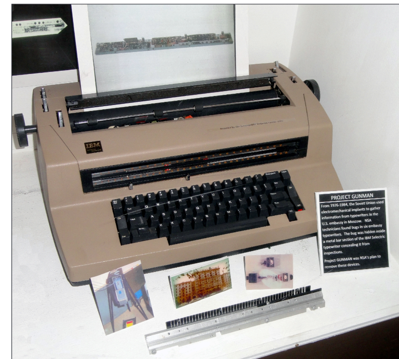
Project GUNMAN exhibit at the National Cryptologic Museum, Ft. Meade, MD, showing the metal bar that concealed the typewriter bug
